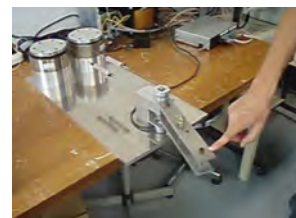
Fig. 3 Stiffness Adjustable Tendon
